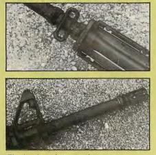
Thicker barrel at muzzle prevents bending.
